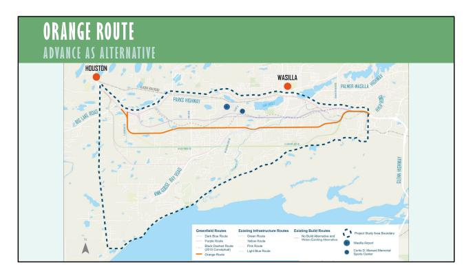
The Orange Route parallels the existing Parks Highway one- to oneand-a-half miles south. This route is a relatively straight alignment with minimal curvature. It uses Fairview Loop Road at the eastern end and joins with Johnson Road after following a relatively straightline connection primarily through undeveloped land.
